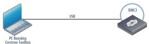
The **USB-OTG** port on the RMC3 connects to the USB port on the PC via the included Type A to Mini-B USB cable:
