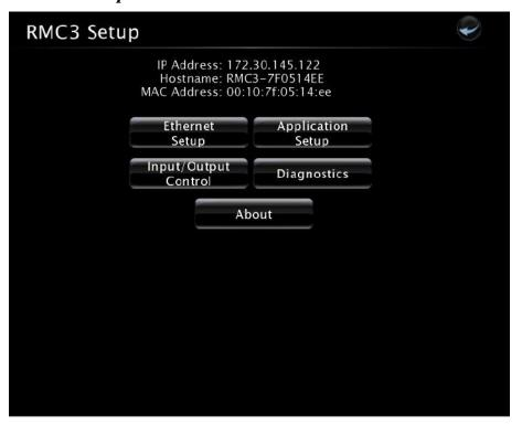
The "RMC3 Setup" menu displays the IP address, hostname, and MAC address of the device. It also allows access to various setup and programming screens. The "RMC3 Setup" menu contains buttons for **Ethernet Setup**, **Application Setup**, **Input/Output Control**, **Diagnostics**, and **About** as shown in the illustration on the previous page.
