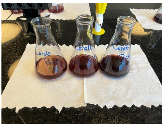
Figure 15: Three samples of Corote Peach after reacting with Eriochrome black T. Elaborated by author.
