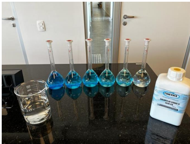
Figure 1: All material used to produce the solutions with a known copper concentration. Elaborated by author.
