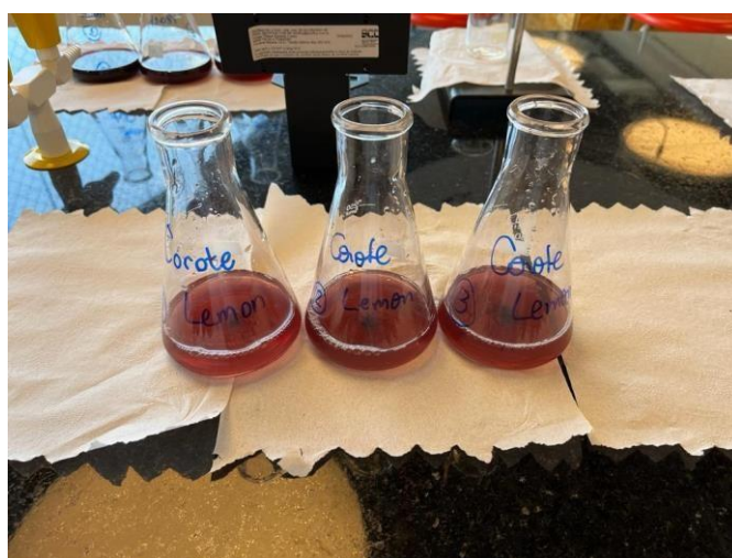
Figure 16: Three samples of Corote Lemon after reacting with Eriochrome black T. Elaborated by author.
