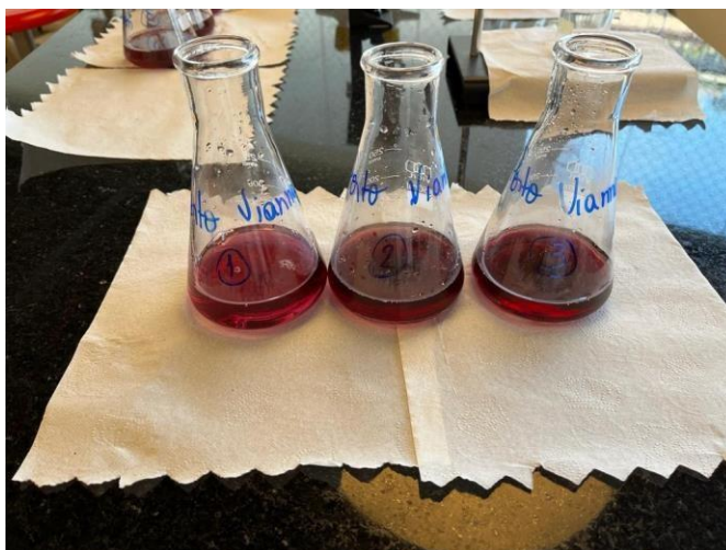
Figure 17: Three samples of Cachaça Porto Vianna after reacting with Eriochrome black T. Elaborated by author.
